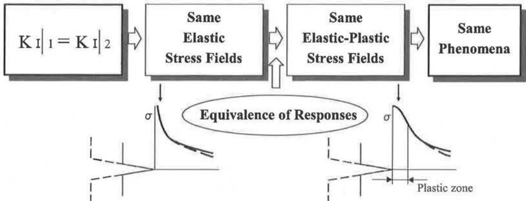
Fig.1 Linear crack mechanics [ 1 : Specimen , 2 : Real Object ].
