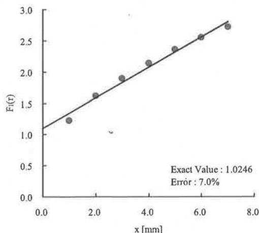
Fig.6 Stress extrapolation method.
